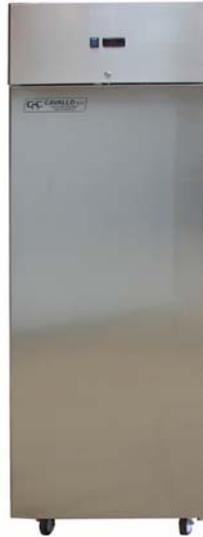
Refrigerated air ventilated Cabinet without electrical contacts inside the chamber, ideal for use with materials releasing vapors. Air Extraction system by centrifugal fan, may be connected to external aspiration. Timer for air exchange inside the chamber. Anti-dust filter inlet.
